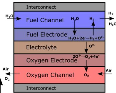
Figure 2: Schematic of SOC model.
