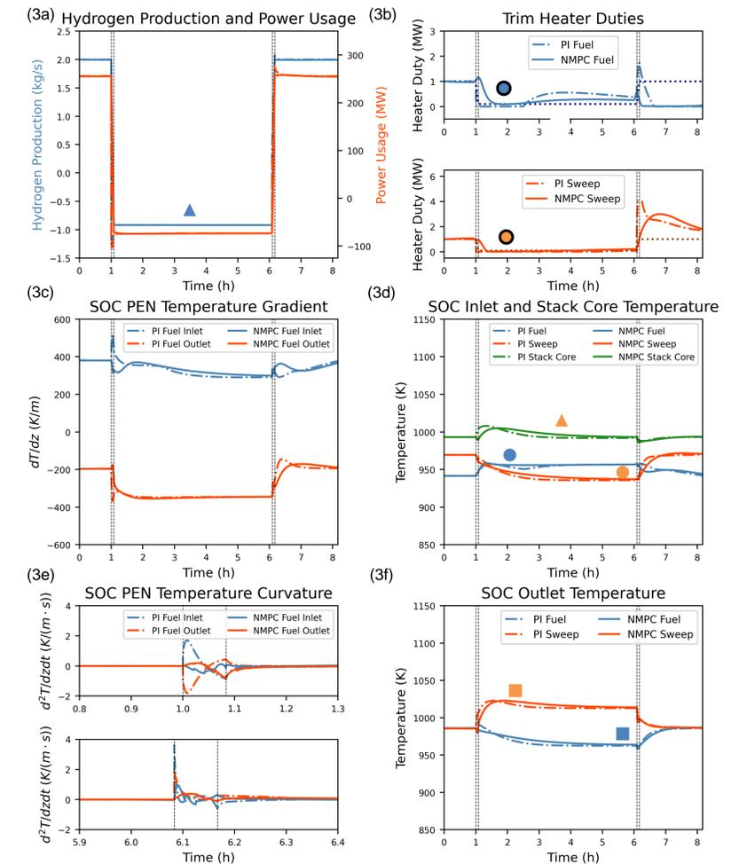
Figure 3: Comparison of classical control with NMPC
