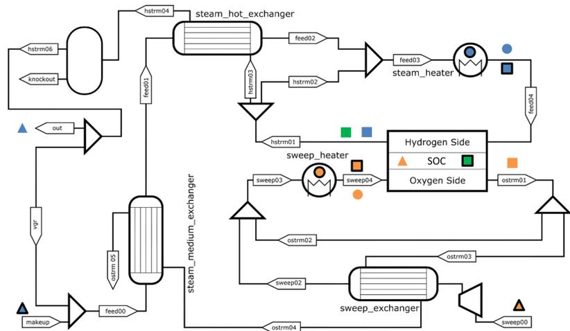
Figure 1: Process flow diagram of SOC system.
