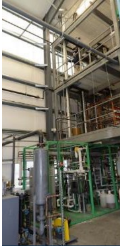
RTI Large Bench-Scale System (2014-2016) Demonstration of key process features ( \leq 2,000 kJ/kg CO 2 ) at bench scale
