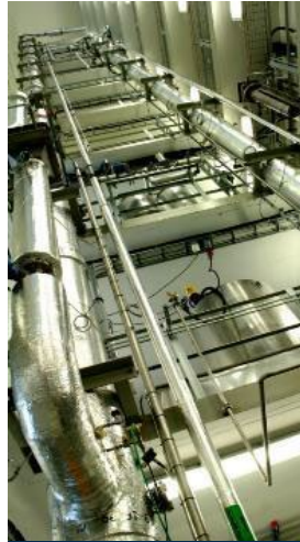
SINTEF Pilot Testing at Tiller Plant (2015-2018) Demonstration of all process components at pilot scale with real flue gas
