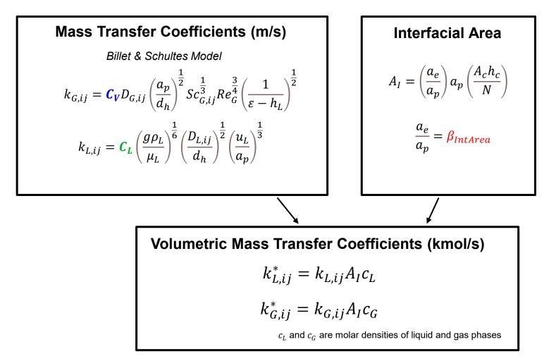
New interfacial area model being developed by PNNL that is a function of physical properties and can be tuned to different types of packing
