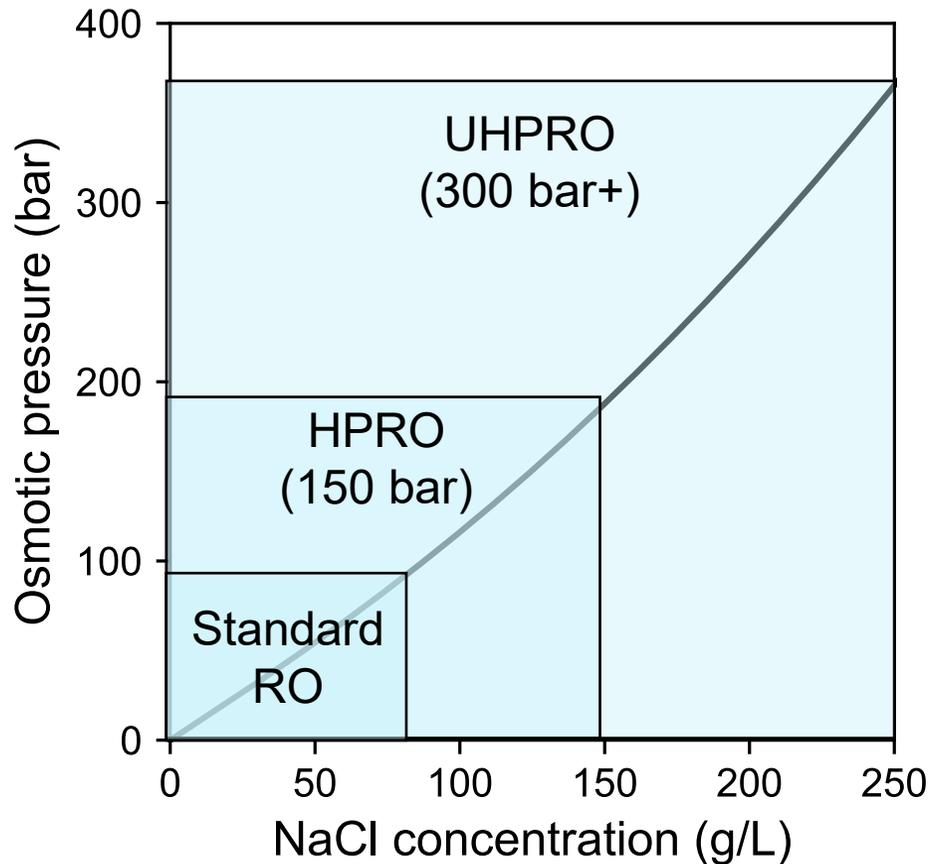
Membrane performance degrades with increasing pressure!
